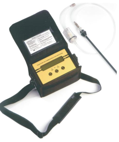
**TRAK-IT®III CGI** with its durable design and easy operation will make finding gas leaks fast and accurate. The bright LCD display shows all gas concentrations simultaneously fulfilling any confined space entry requirements. A bar-hole test button helps accurately locate below ground leaks. High resolution display (0.1% LEL) in combination with the high volume rotary pump helps to quickly locate hard to find leaks.
